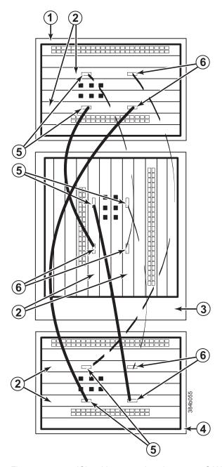
Figure 48. 3-way ICL cable connections between a SAN768B chassis and two SAN384B chassis.
